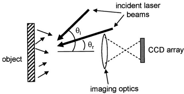
Fig. 3. An electronic speckle pattern interferometer using a simplified optical arrangement. Although this arrangement eliminates the need for a complex optical system, it results in reduced sensitivity to out of plane displacement.
