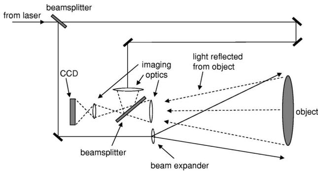
Fig. 1. Schematic of an electronic speckle pattern interferometer that is sensitive to out of plane displacement.
