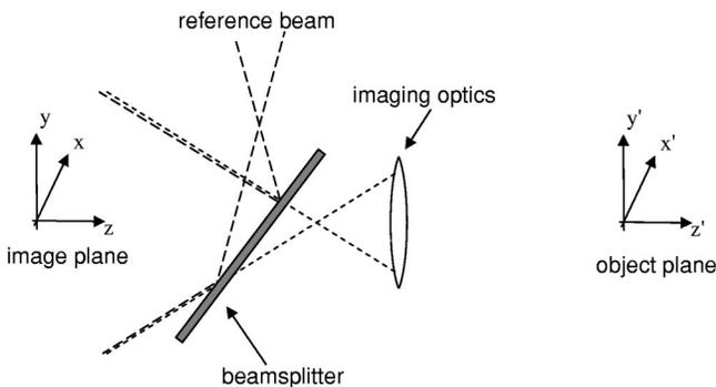
Fig. 2. Simplified schematic of the optical system of an electronic speckle pattern interferometer. Coordinates in the object plane are designated by primes; the image plane is in the unprimed coordinate system.
