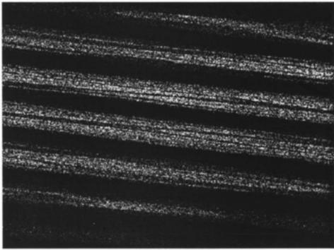
Fig. 5. Interferograms of a 17 cm circular plate vibrating in one of its normal modes. Theoretically the two modes occur at the same frequency, however, the degeneracy is broken by a slight asymmetry in the plate. The frequencies of vibration are 2133 and 2145 Hz.
