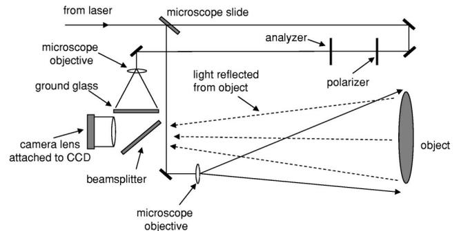
Fig. 4. Schematic of an electronic speckle pattern interferometer that does not require a complicated optical arrangement but does not have reduced sensitivity.
