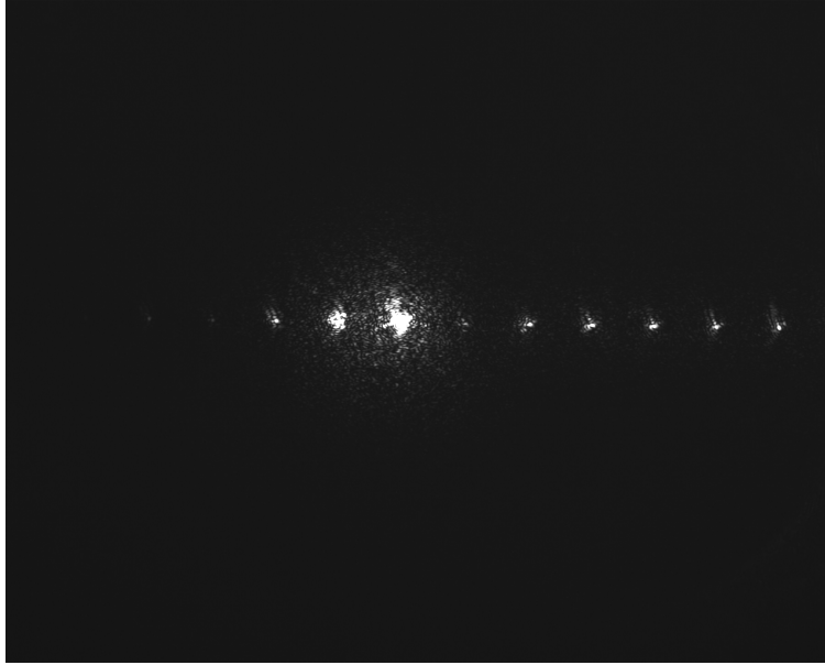
FIGURE 4.5: A diffraction grating was placed after L1, with L2 removed from the system, so that collimated light was incident on the grating. Light was redirected by the grating at various angles, and that light was collected by the MO. The irradiance maxima, called orders, occurred at angles which could be calculated from the diffraction grating equation, 4.1.
